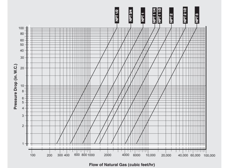
Flow Curve Using Natural Gas for class II regulator.
