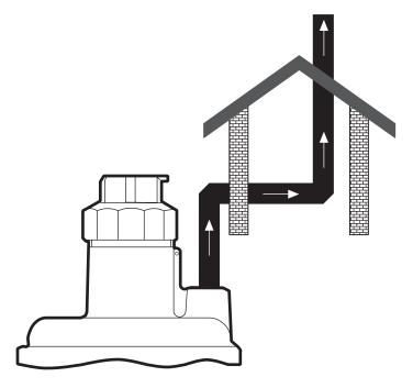
In the absence of venting codes and where venting is required, each regulator must be vented separately from all other vents.
