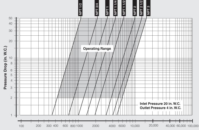
Flow (CFH) of natural gas; s.p. 0.65 at 60°F
