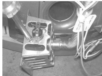
Step 7. Place new resettable thermal switch in place. Be sure contact surface of resettable thermal switch and manifold mount are free of any debris. Secure resettable thermal switch into place using screws from step 6. **DO NOT OVER TIGHTEN SCREWS.**
