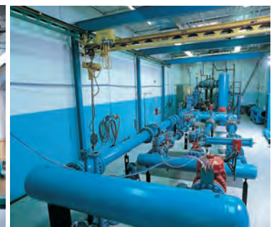
High Pressure Flow Loop; up to 900 psi (62 bar)
